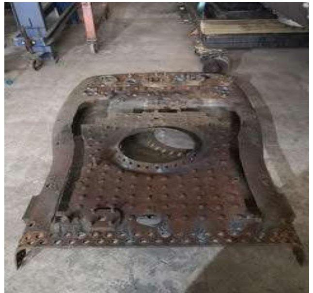
The old back head lying on the floor of the HBSS workshop.
