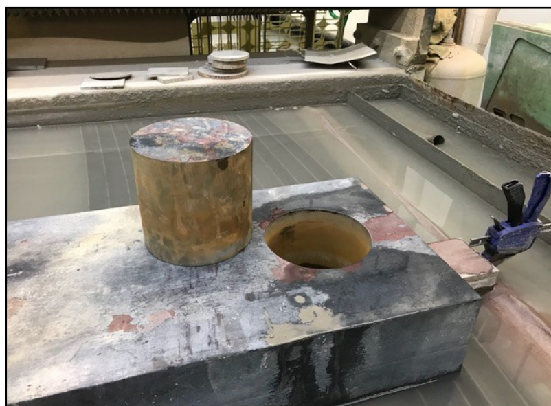
First to be cut — the holes for the crank pins!
