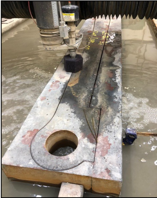
The shape of the rod begins to appear on the water cutting bed.
