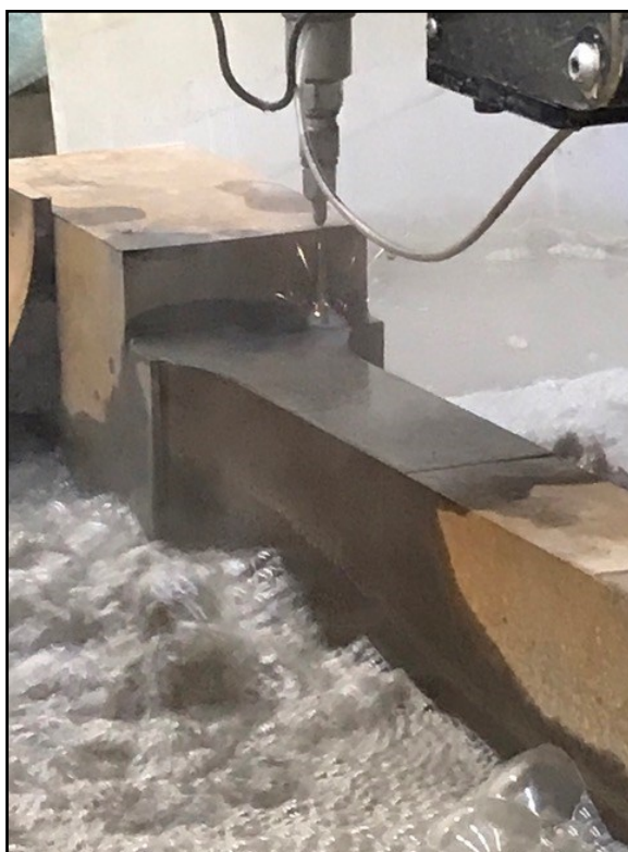
Here you can see the water jet in action, cutting along the side of the billet.
