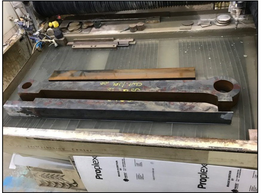
The billet lying on the now-drained cutting bed after the side cuts have been made.
